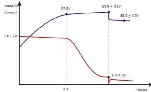
**Phase 1:** The Max. charge current is 5A, and the charge voltage is gradually risen up to 57.6V;
